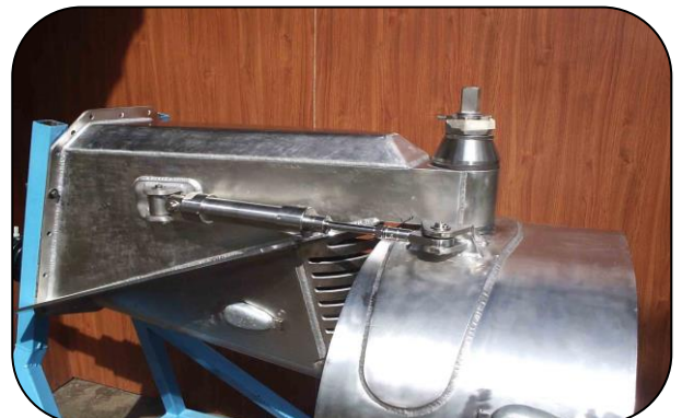
LD 280-300 with hydraulic steering
