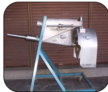
LD 240-250 with hydraulic steering
